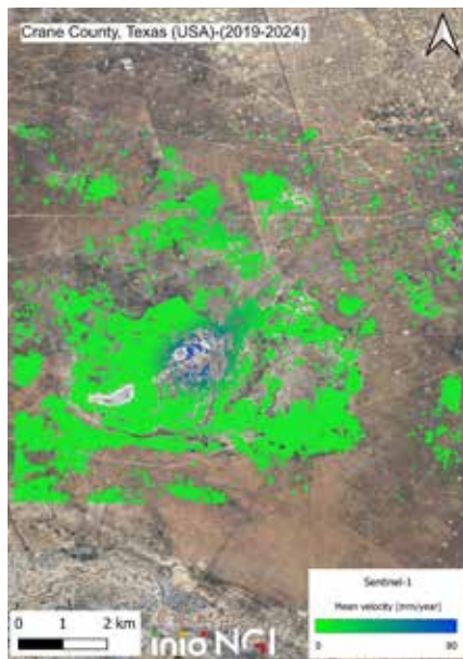
Figure 3. Application of DInSAR analysis for detection of surface movement due to saltwater injection, in the wells, in Crane County, USA. The blue colour indicates uplift, whereas the green areas can be categorized as stable (Image credit: NGI).
