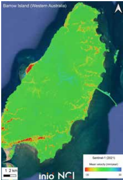
Figure 2. Example of SBAS DInSAR application in oil-gas barrow, Island; Australia. The blue color shows uplift, and the red color refers to subsidence. The green color shows relatively stable area. (Image credit: NGI)
