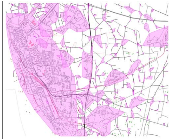
Figure 5. Clusters created with minPts=7 and \epsilon=115m . Max length of line segments is 200 m
