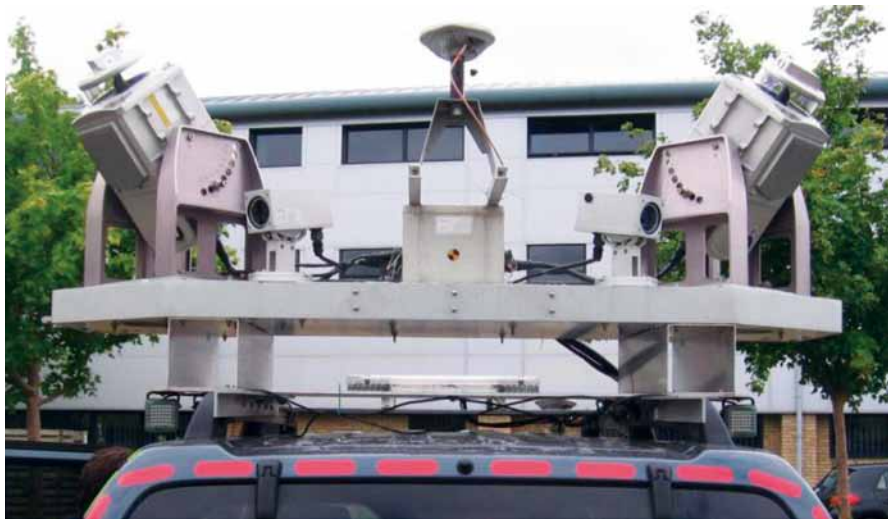
Optech Lynx 200 mounted on top of a Nissan Pathfinder
